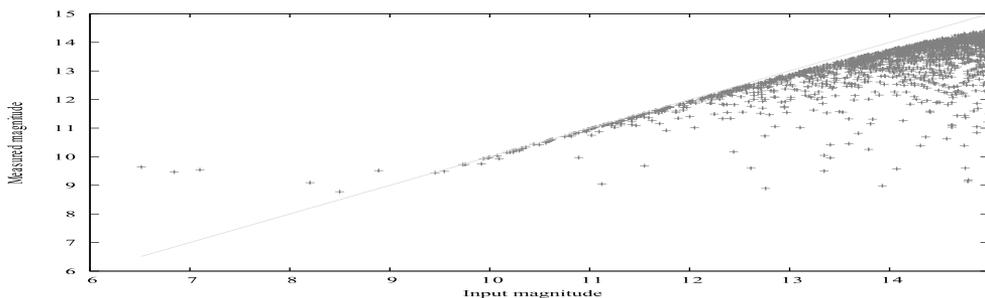
**Fig. 3.** Magnitude of the stars in the generated synthetic images as measured with the photometric process as a function of the input magnitude given in star catalogue. The green line indicates the measured magnitude equal to the input magnitude.
