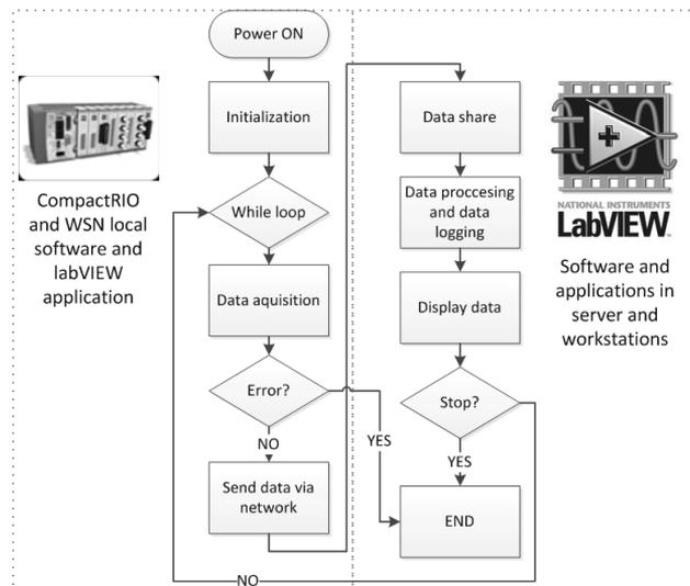
**Fig. 4.** The flowchart of data acquisition system
