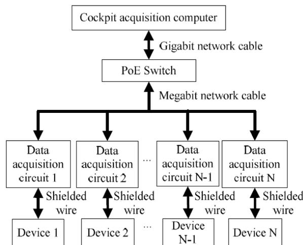
**Fig. 2.** The topological structure of distributed data acquisition using embedded Ethernet and Power over Ethernet (PoE) technology [5]
