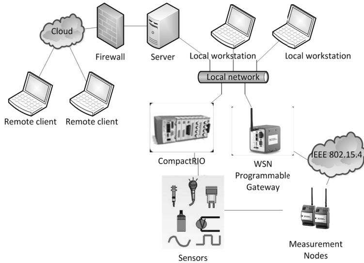
**Fig. 3.** The proposed topological structure of the distributed real time data acquisition system
