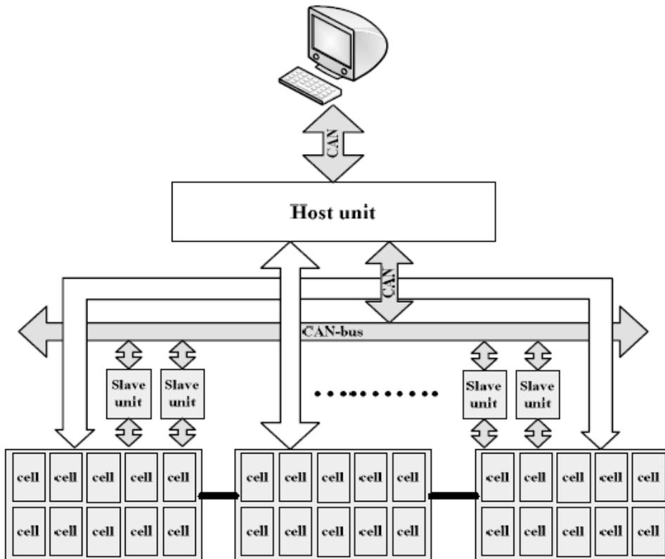
**Fig. 1.** The structure of the distributed data acquisition system [4]
