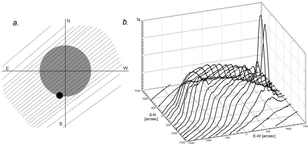
**Fig. 1.** *The tracks of the Sun's azimuthal scanning telescope on 2012, July 17 UT 7:15 in relation to the center of the Sun and the Sun's axes. The black spot presents the antenna HPBW(a) at the 3.76 cm wavelength. The set of 1D scans of the antenna temperature (b)*
